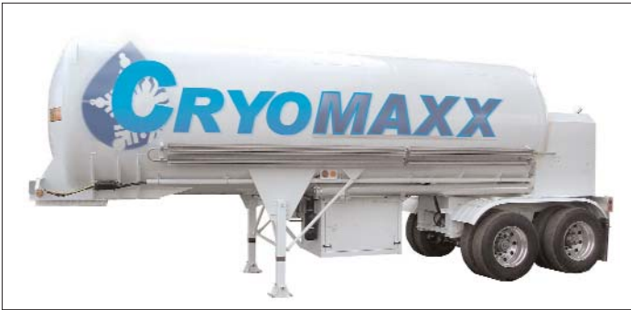
Acme Cryogenics recently developed this self-contained trailer system, the Cryomaxx CM-4600, which has a gross water volume capacity of 4600 gal, yet only a 25-foot overall length, combining good maneuverability, plenty of capacity and reduced operating expenses.
