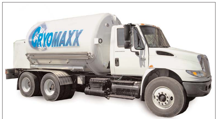
Microbulk was developed nearly 20 years ago to help major gas suppliers make deliveries into tight areas, make smaller drops in densely populated places, and eliminate cylinder handling. Pictured here are Taylor-Wharton’s newest Express III cryogenic microbulk delivery system truck and Acme’s CryoMaxx Liquid Microbulk delivery vehicle.
