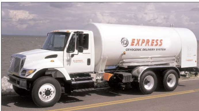
Microbulk was developed nearly 20 years ago to help major gas suppliers make deliveries into tight areas, make smaller drops in densely populated places, and eliminate cylinder handling. Pictured here are Taylor-Wharton’s newest Express III cryogenic microbulk delivery system truck and Acme’s CryoMaxx Liquid Microbulk delivery vehicle.
