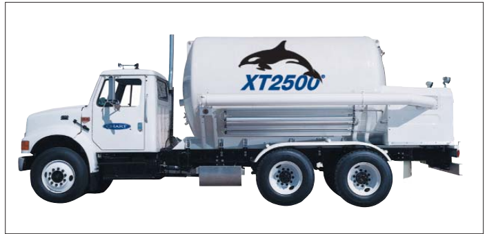
Chart plans to begin production in 2007 of the XT2500, a new larger pump-less system based on its pulse technology introduced in 2005. The new system, under final development, utilizes a small 300-liter pod connected directly to the primary storage vessel. "
