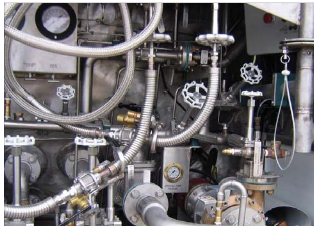
A dual-hose configuration is standard on Taylor Wharton's Express Delivery Systems and allows the gas distributor to fill both traditional smaller Microbulk tanks and larger Microbulk tanks as well as small standard bulk tanks from the same Express truck.
