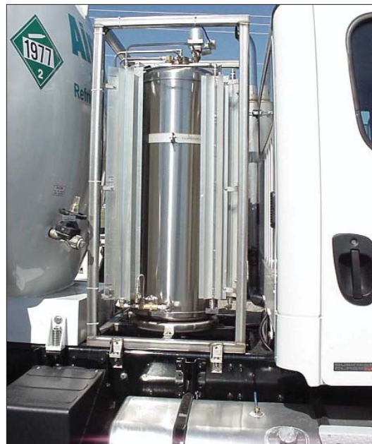
A delivery-assist option that became available from Chart late in 2004 allows the distributor to hook up the customer's laser-cutting-system supply line directly to an assist cylinder mounted on the Orca delivery unit while the driver depressurizes and refills the customer's Perma-Cyl.
